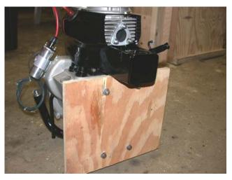
Using a minimum of 6 (3 on each side) 3" long decking screws attached the engine mounting board to the 2-1/4" high boards mounted in one end of the crate.
