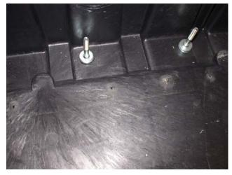
Complete the securing of the 31" boards by placing a flat washer and nut on top of the board and tightening securely.
