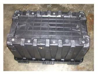
Have an assistance hold in place one of the 31" 2"x4" boards in either the front or rear of the box on the inside. Mark the holes on the board using a pencil. Drill 3/8" holes through the 2"x4" at the locations marked. Do the same for the opposite side.
