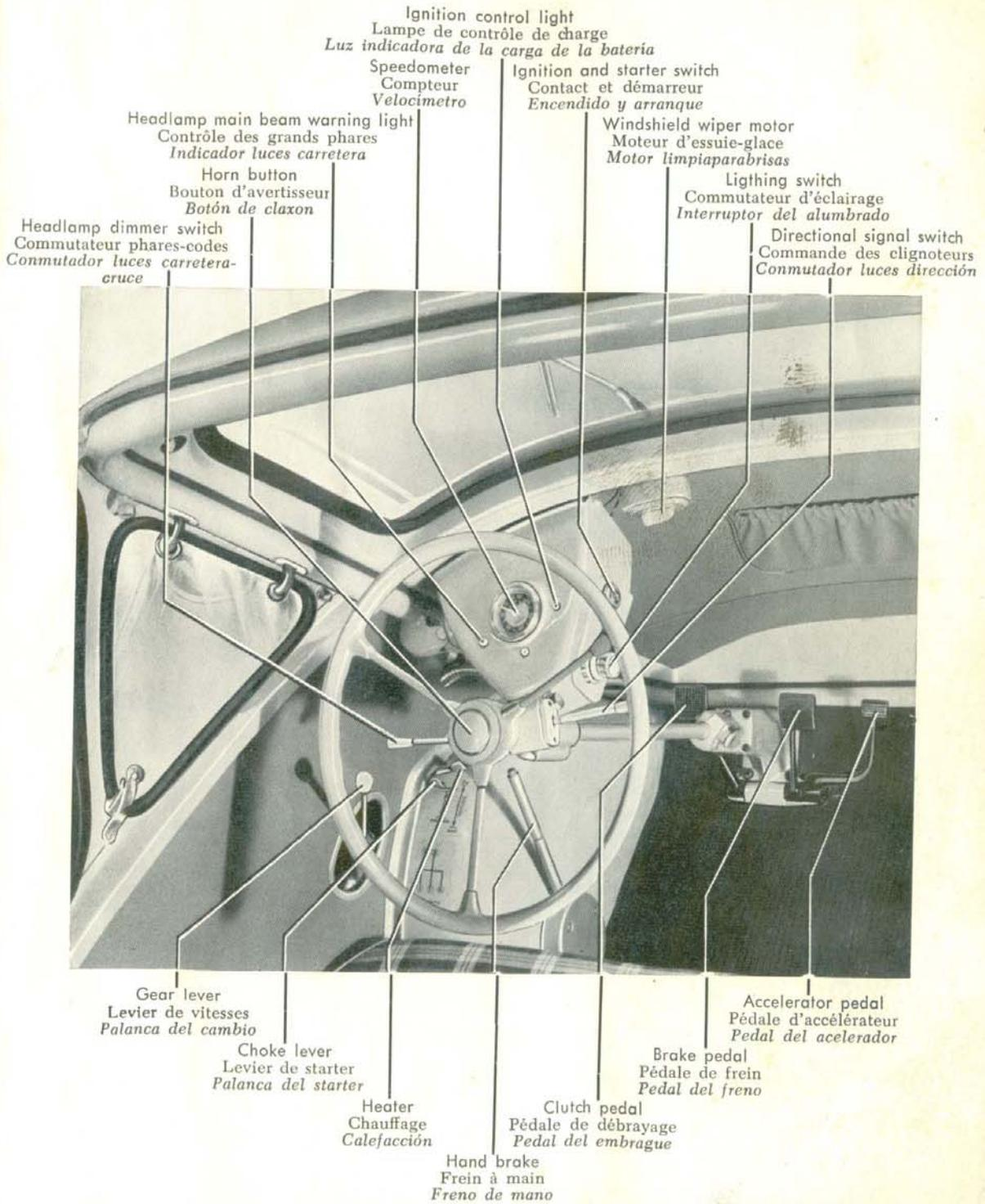
Direction indicator warning light (green light) is situated below the speedometer
