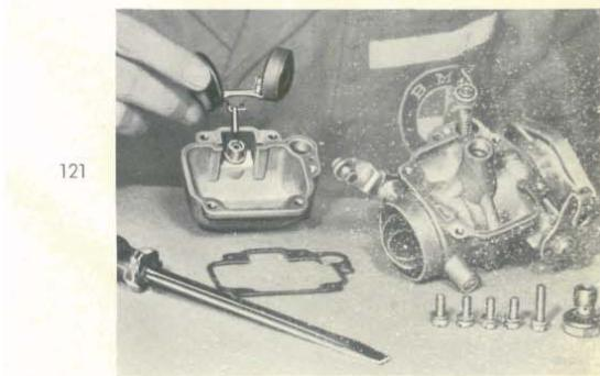
9. Loosen hollow screw SW 17 on fuel union body and remove the two parts together with the corresponding two gaskets.
