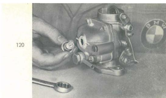
7. Remove main jet from carrier by means of screw driver. Remove bowl with gasket from air-intake body. For this purpose remove four short cylindrical screws from the bowl and one long cylindrical screw from the air intake body together with their lock washers by means of a screwdriver.
