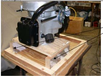
Install the (2) 2"x4"x11" boards in the corners of one end of the box as shown. The 4" height of this board must be at least 4" (not 3-1/2").
