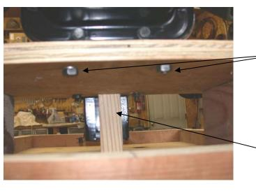
Secure the engine to the 3/4" plywood with the engine mounting nuts and washers (four locations)
