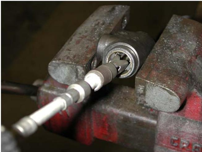
On the larger front cylinders, use a cylinder hone to clean up any burrs on the cylinder wall from the drills. Also make certain you clean the edges where you used the dermal tool to dress down the ends of the brass tubing.
