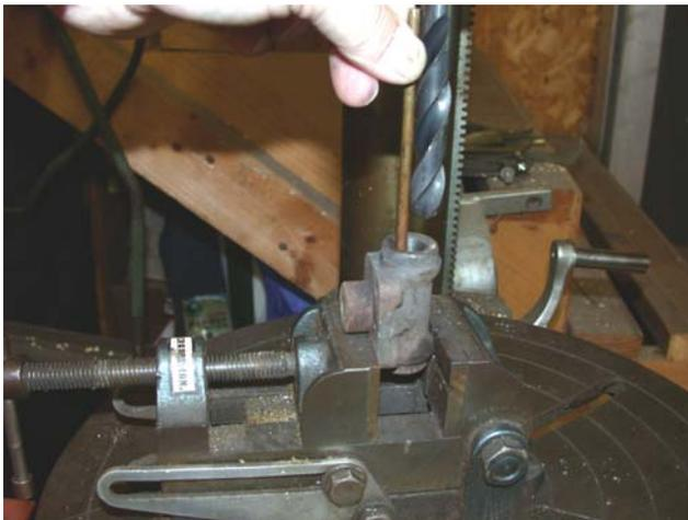
Use some type of straight edge and make sure the cylinder is true with the drill. Check the squareness in both the "X" and "Y" axis. After you are certain all is true bolt the vice down to the drill press (if possible). This last part is not completely necessary, but it does afford you some safety in the event the drill catches in the cylinder.
