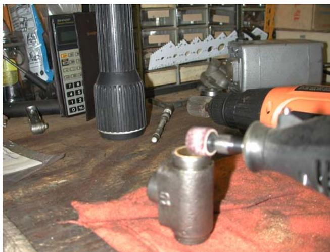
After the cylinders have set for at least 24 hours, dress off any excess brass with a dermal tool.
