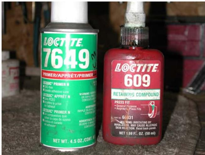
Using Loctite cleaner-primer, prime both the inside of the cylinder and the exterior of the brass tube. Allow the primer to dry as instructed on the container.
