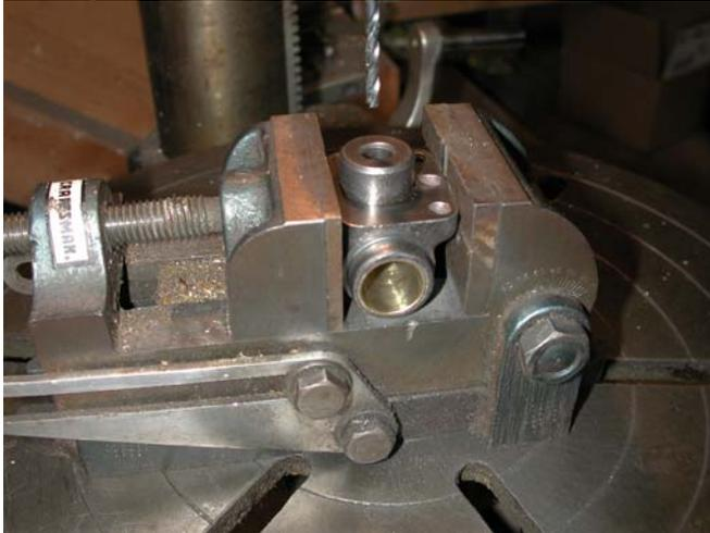
Using a number 28 drill, drill the hole for the hydraulic supply fitting.
