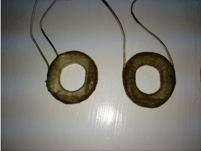
New generator field coils for Dynastart
