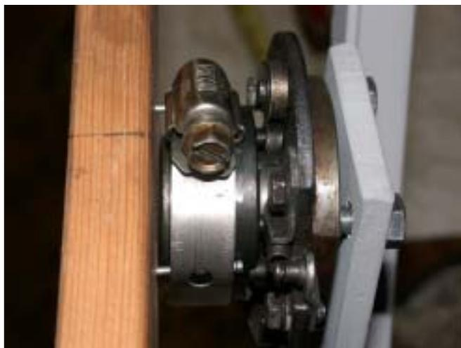
Prior to tightening the clamp completely, make sure the advance is in the full retard position. Adjust the board so that it is at an 11 degree incline as show in the picture on the next page. Full advance on the unit is 22 degrees. This will allow mid-advance to occur with the board exactly level.
