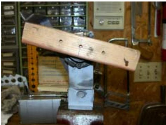
Now either using weights (on the left) or a spring gauge (on the right as shown in this document), check the amount of weight it takes to move the board to the "level" or 1/2 advance position. This should be approximately 3 oz.
