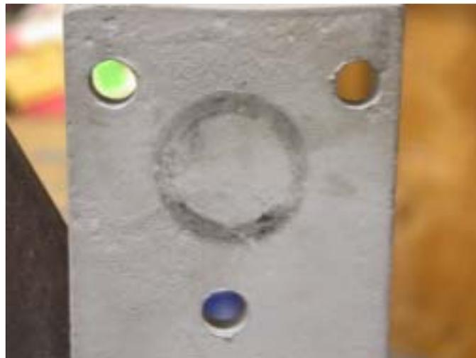
With the bracket mounted in a vice I bolted the advance unit to this bracket using (3) 6mm x 15mm cap screws.
