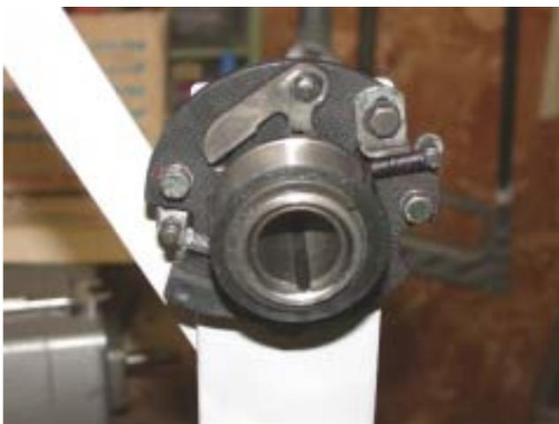
Using an appropriate size hose clamp, clamp the board with the two finishing nails to the cam part of the advance. Be careful not to allow the wooden board to drag on the center of the advance which does not rotate.
