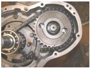
With the chain in position around the camshaft sprocket, wrap the chain around the crankshaft sprocket and bring the two ends together. Install the link and the chain tensioner and you will have a perfectly timed camshaft!
