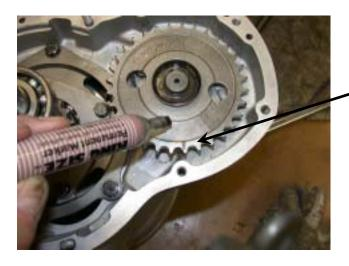
Mark one tooth on the gear for a reference point.
