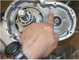
Install the chain on the sprocket and rotate the sprocket clockwise until you return the sprocket to its marked position. Be sure to start the chain about four to five links beyond the "marked" tooth.
